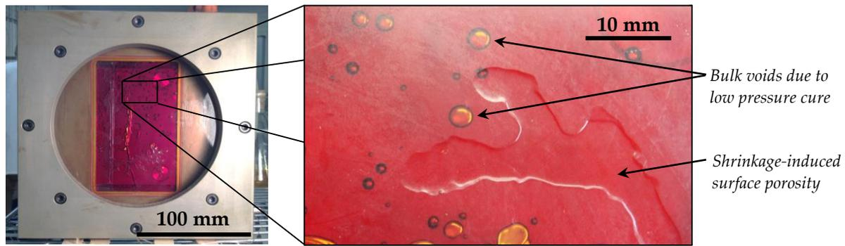
**Figure 1:** Lab-scale RTM with neat resin sample cured at low pressure, containing both types of voids.
